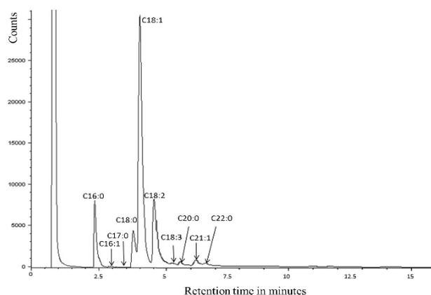
Figure 1. GC chromatogram showing fatty acid profile of extracted cashew nut oil
